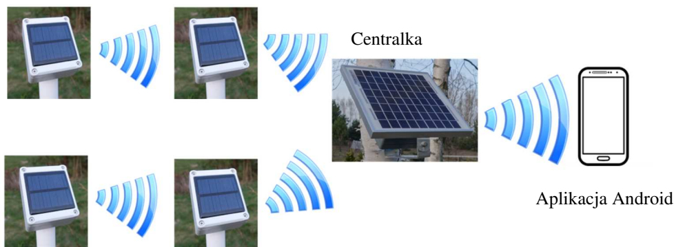
Rys. 6. Schemat systemu Aquastatus Fig. 5. The scheme of Aquastatus system
